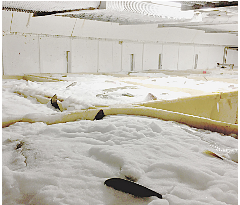
Fish are placed in containers filled with slurry ice and seawater where they bleed and cool very quickly before being placed in a second container with other fish and thin layers of liquid ice. Photo courtesy of KAPP.
