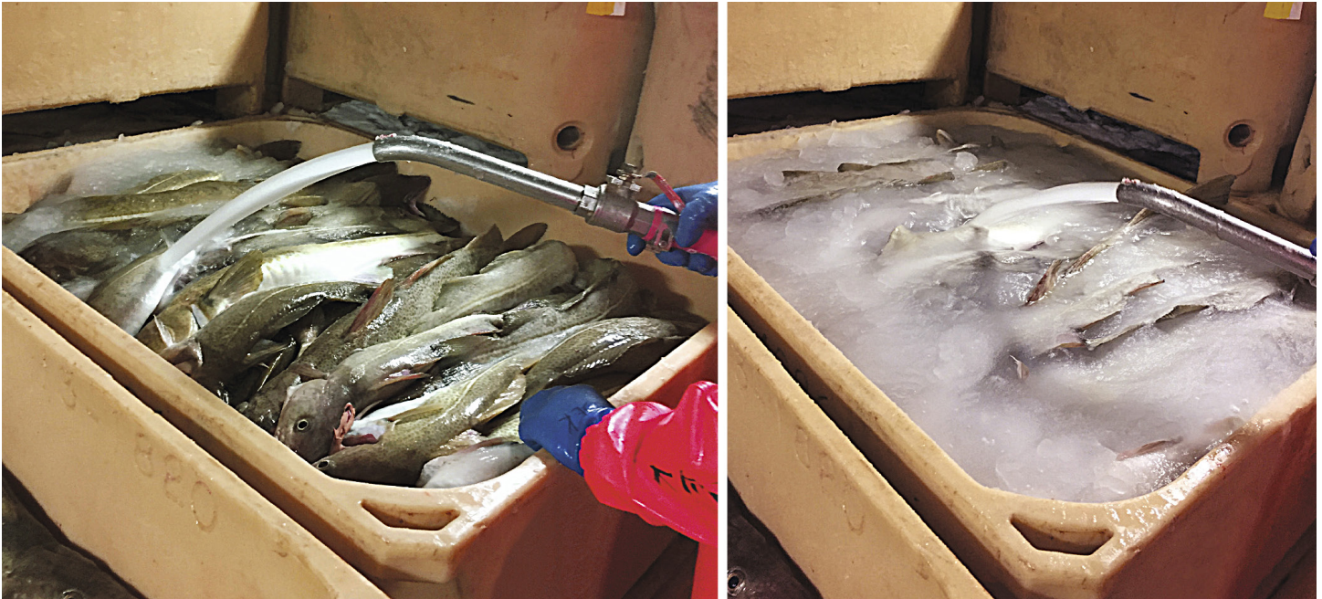
Instead of having to shovel ice, Icelandic fishermen can apply slurry ice through a hose, and spread it over the fish. Photos courtesy of KAPP
